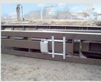
The joint inspector has been designed in modular units and is easy to mount to the steel frame of the grab unit. Up to 5 sensors can be implemented.
