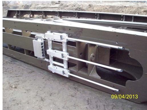
Picture 10: Modular units of the “joint inspector” in full set up
